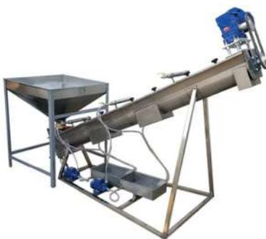
Screw conveyors are in two models, angled/vertical and horizontal model. Also they are made of stainless steel, galvanized or painted steel. With installing high pressure water nozzles on conveyors, these machines used for washing.
