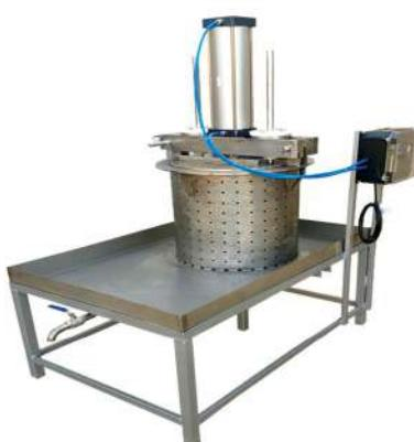
Extractor can be used manually or pneumatically and hydraulically for extracting dates or some fruits or oil from sesame waste.
