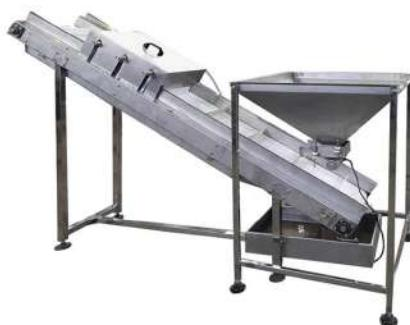
Belt conveyors used for a variety of materials with PVC or modular belt in food industry. It is also possible to install water nozzles for washing.
