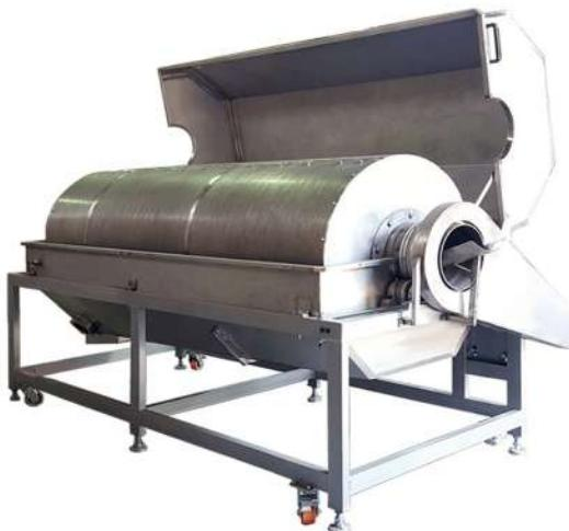
Blancher is used in the canning industry for the production of canned chickpeas, carrots, corn, etc. also it used for nuts Pre-peeling.
