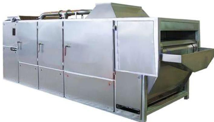
Belt roasting machine has advantages of fast roasting speed, high evaporation strength and good product quality, for the oilseeds. Cooling unit is another advantage of this machine.
