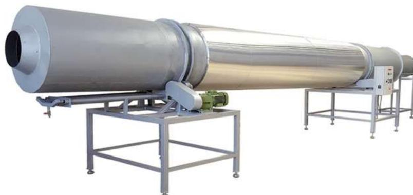
Dryers capacity depends on burner capacity and their Length and diameter .
